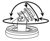
Move the camera along its 3 axes to adjust the pan, tilt, or rotation.
